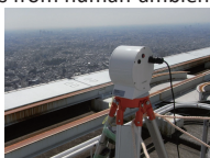
■ Estimation of heat fluxes using Scintillometer
