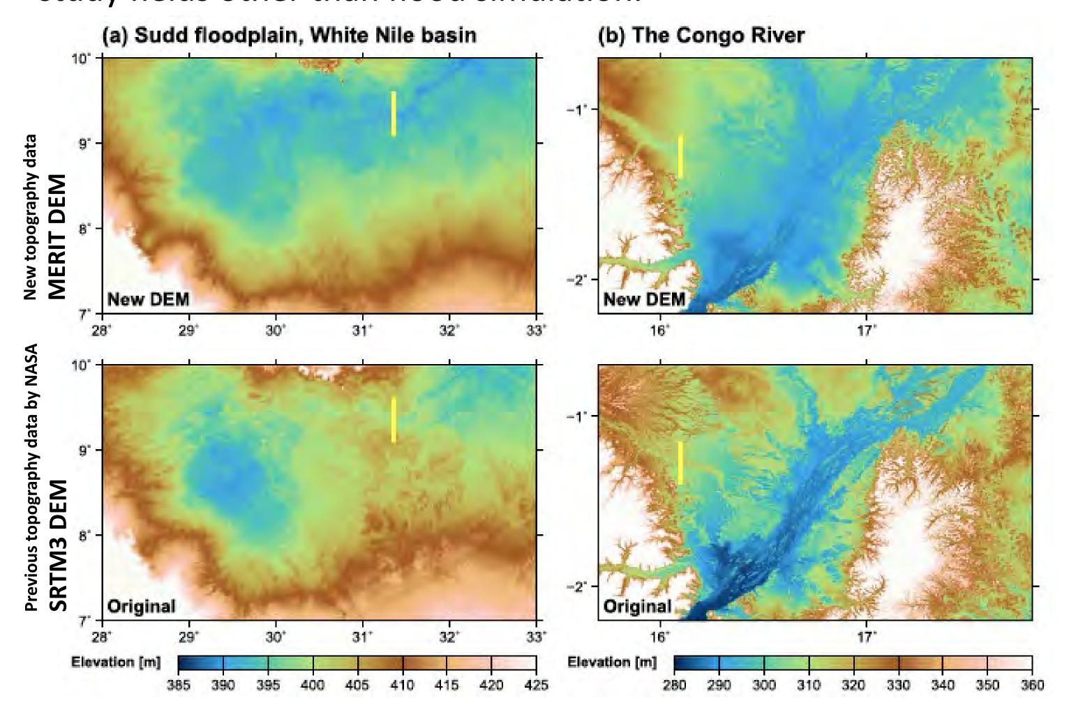
MERIT DEM: A precise topography by multi-component error removal High accuracy topography map was developed by combining multiple satellite data and The first world map of river width, based on the removing multiple error components. Now widely used in various research fields. satellite-derived high-resolution water body data.
