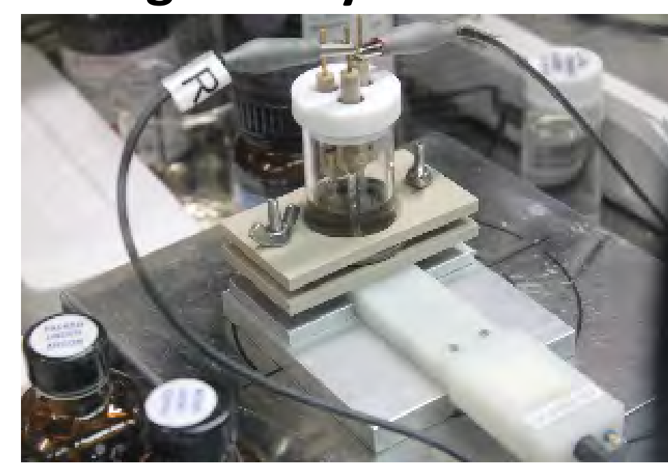
Analysis of the insertion/extraction behavior of Mg ions by electrochemical QCM
