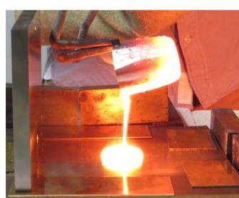
Melting of simulated waste
