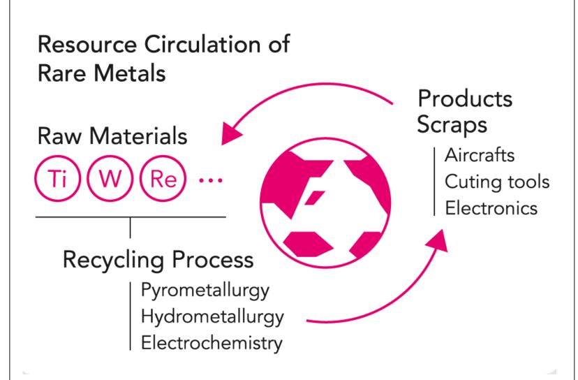
Our laboratory is developing new, efficient and environmentally sound processes to recycle rare metals for which an increase in demand is expected, such as titanium, tungsten, cobalt, rhenium and platinum group metals.
