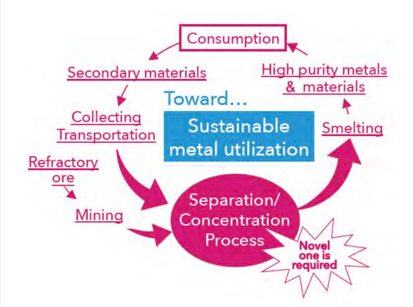
In our laboratory, solid / solid separation and concentration technology without heating / dissolving the waste or refractory ore is studied to achieve an energy-saving separation and concentration process. This process is regarded as "pre-treatment" or "middle treatment" before metallurgical / hydrometallurgical process, which produces high-purity metal.
