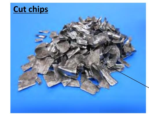
Fabrication of aviation parts using Ti alloys usually involves a material loss of up to 80-90 %.
