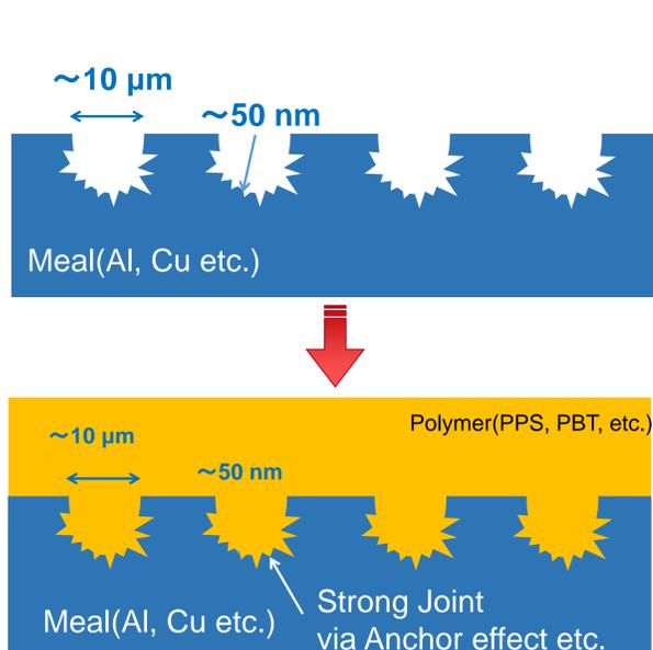
Fig.4 Metal-polymer hybrid joining
