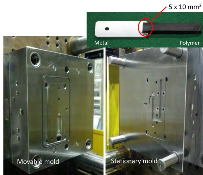
Fig. 5 Mold for joining and metal-polymer hybrid
