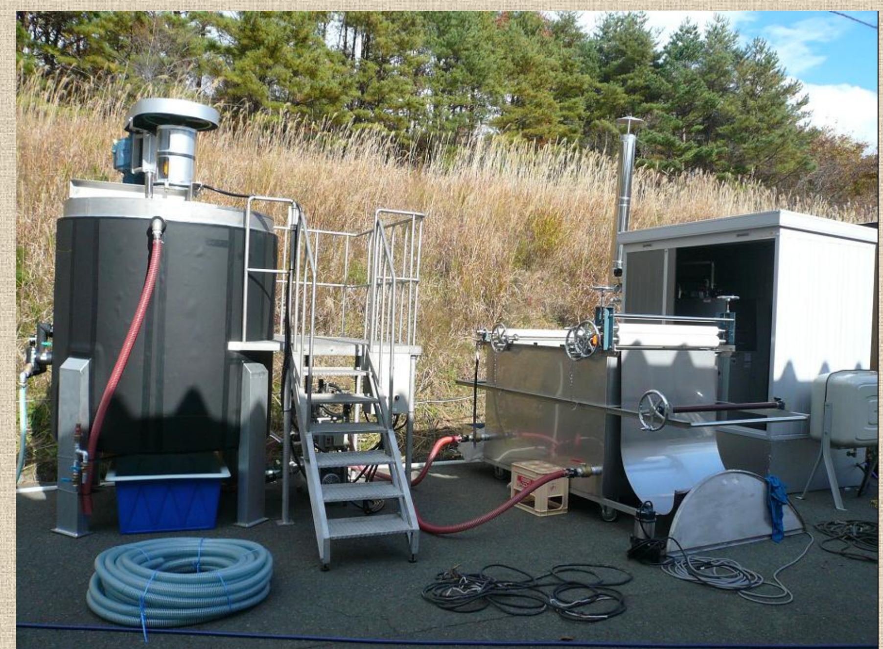
Demonstration of decontamination using a Prototype equipment (Throughput: 2ton-soil/batch)
