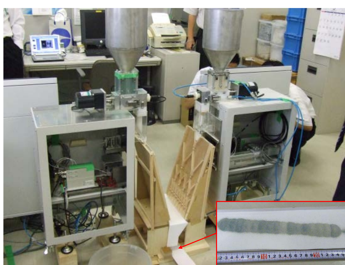
3D mixing system of powder using dividing channel, and mixture of \text{Al}_2\text{O}_3 and SiC.
