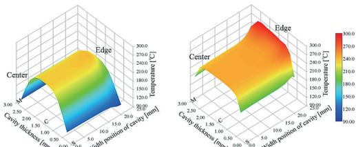
(a) Injection rate 10cm³/s (b) Injection rate 100cm³/s
