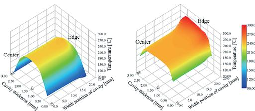
(a) Injection rate 10cm<sup>3</sup>/s (b) Injection rate 100cm<sup>3</sup>/s
