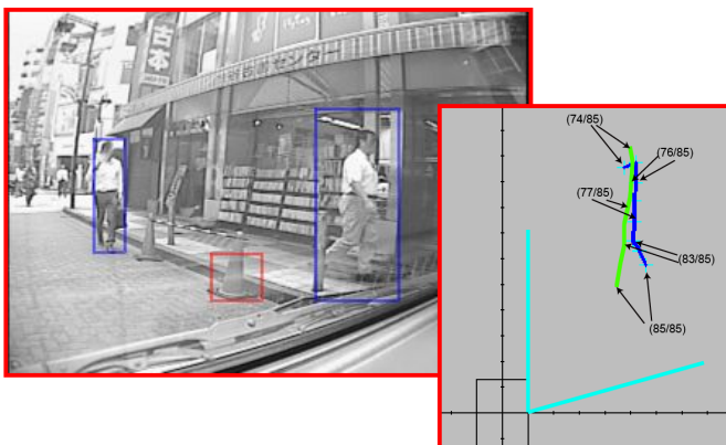
Pedestrian detection by monocular camera
