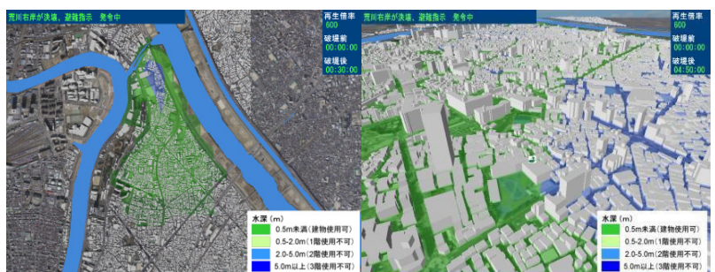
Fig.5 System for Imaging Human Evacuation in Case of Urban Flood
