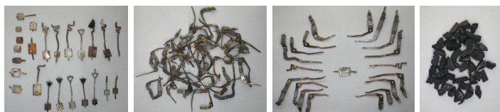
Metals in side Connector metals Metals inside Plastic cover Various Materials Liberated by Electrical Disintegration
