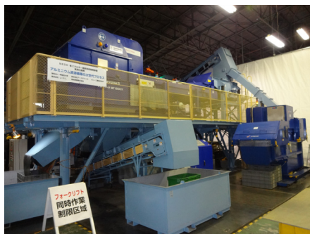
“Sash to Sash” Pilot Plant using XRT·XRF sorters
