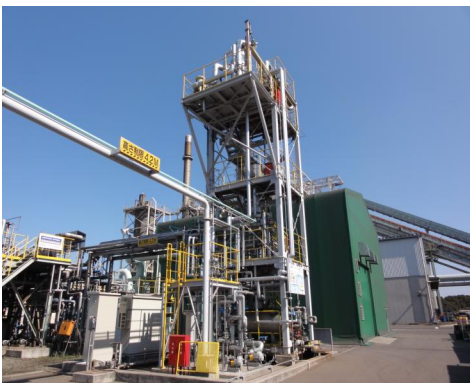
Pilot self-heat recuperative distillation for bioethanol
