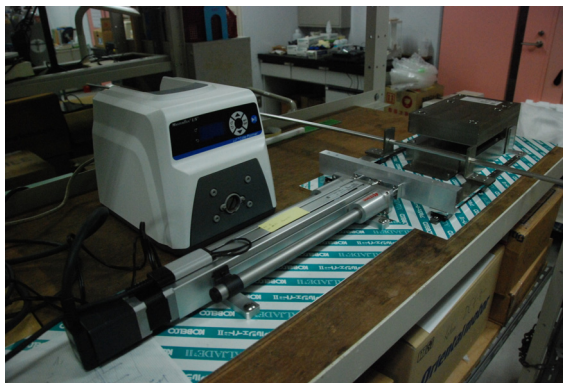
Exergy recuperative experimental device by magneto caloric effect
