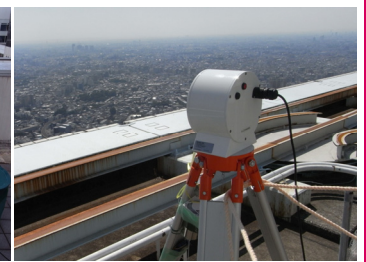
■ Estimation of heat and momentum fluxes using a Scintillometer
