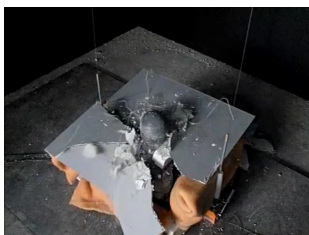
Safety assessment of ceilings by dropping experiments
