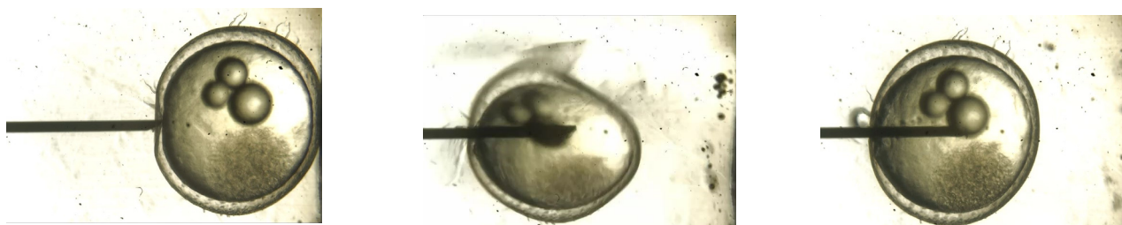
Fig.1 Electropiercing of a fish egg (left: before pulsing, center: during pulse, right: after pulsing)
