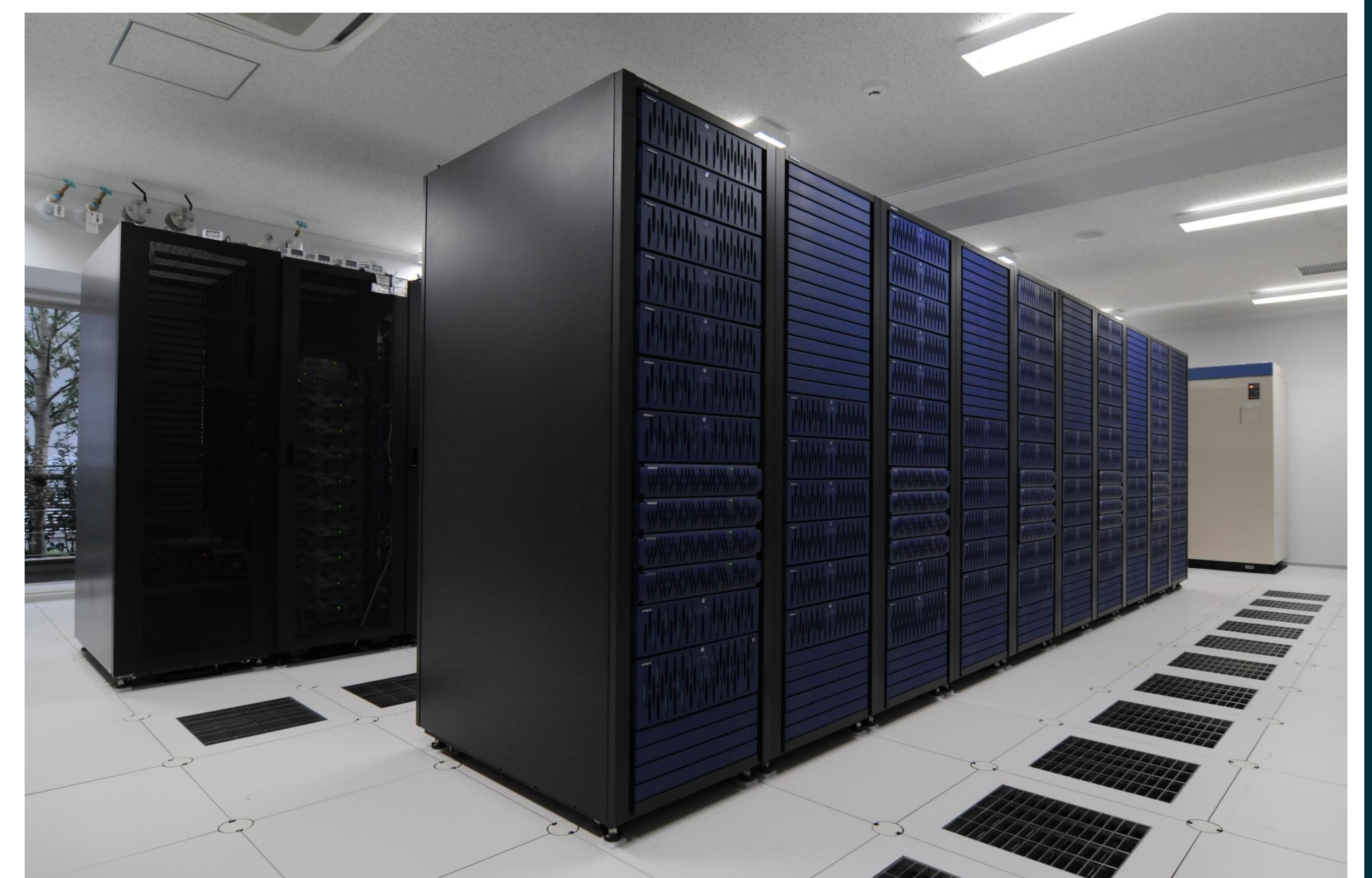
A peta-byte (PB) scale data storage system which store the last 30 years of satellite observation data
