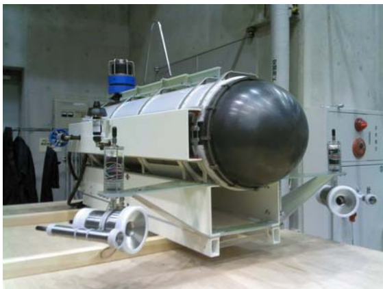
Jellyfish Catcher AUV of 7,300m depth capability with ceramics hull, under development in cooperation with Ura Lab. and Maki Lab. (Length: ab. 1.7m)
