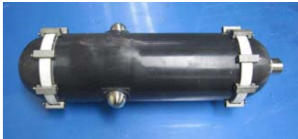
Scale Model of Ceramic Pressure Vessel for 11,000m depth capability (Length: ab.40cm)
