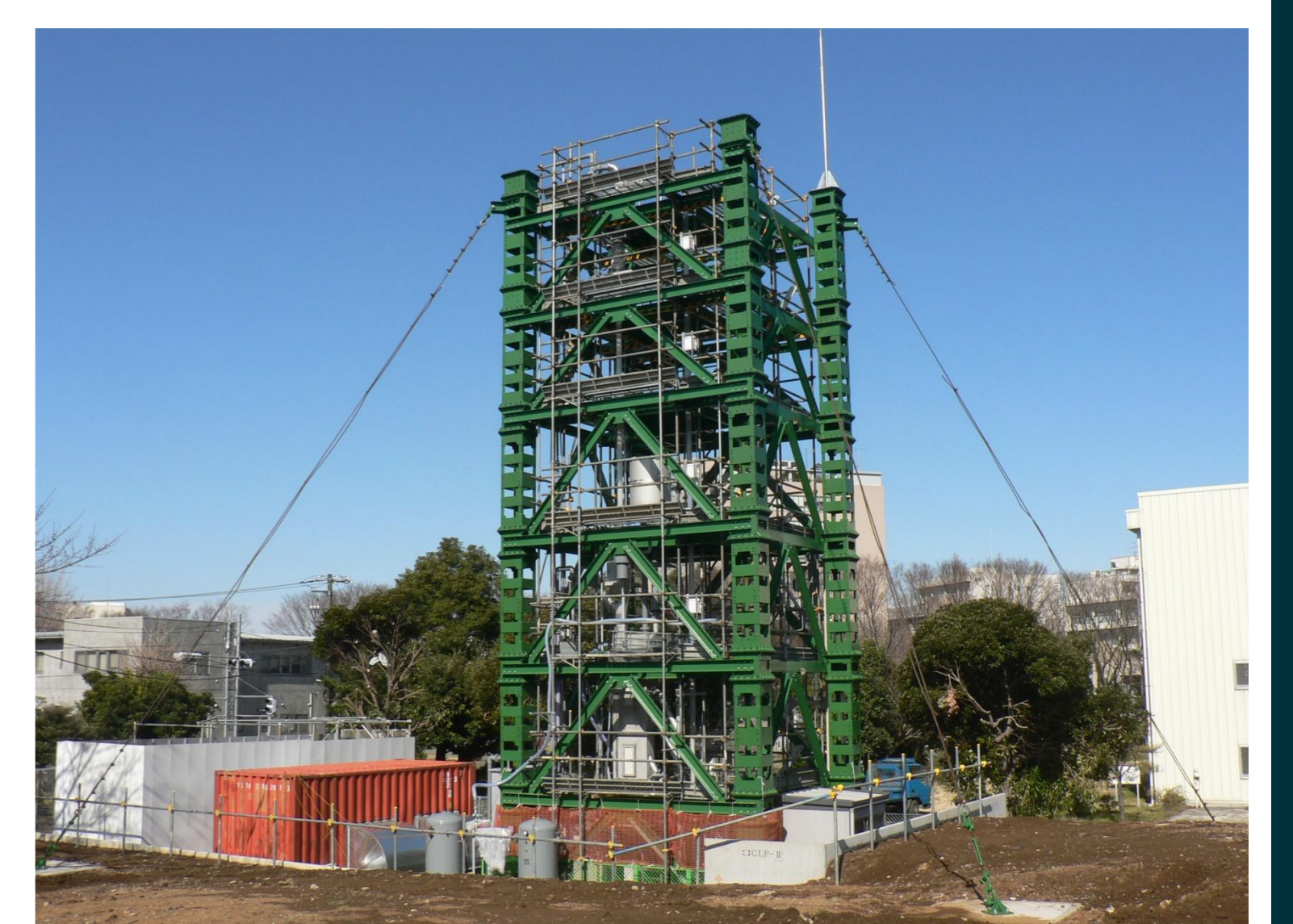
Large scale circulating fluidized bed cold model in Chiba Experimental Station (h: 16 m, d: 0.10 m)
