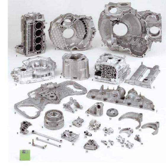
Automobile parts by aluminum die casting
