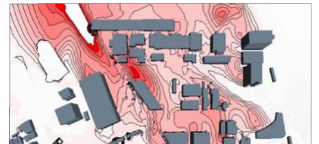
■ Analysis of heat-island effect by anthropogenic exhaust heat using CFD coupled with radiative analysis
