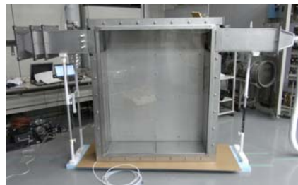
■ Dispersion Experiment of Concentration Fluctuation in Urban Canyon
