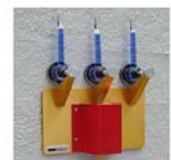
Water permeability test
