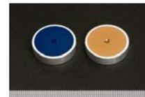
Al alloy machine components coated by the DLC films. The different colors are originated from the interference based on the film thickness, indicating the optical transparency of the DLC.
