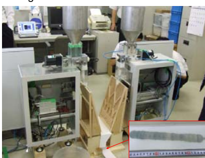
3D mixing system of powder using dividing channel, and mixture of \text{Al}_2\text{O}_3 and \text{SiC} .
