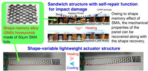
Bending shape can be controlled effectively by uniform application of shear recovery force from Honeycomb to CFRP skins.
