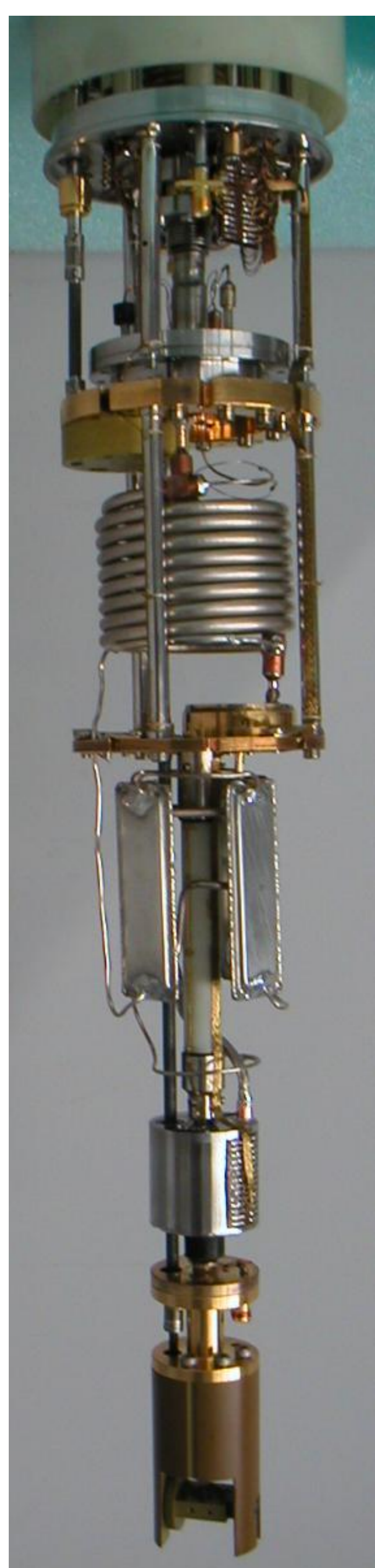
10 mK Dilution refrigerator
