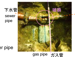
Road cave-in due to corrosion of sewer pipe
