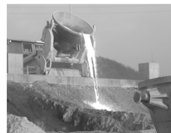
Gradual cooling of steelmaking slag
