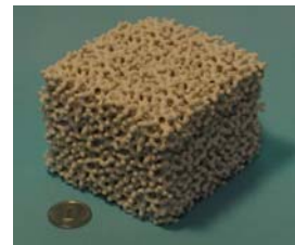
Fabrication of photonic amorphous diamond structure in a microwave regime
