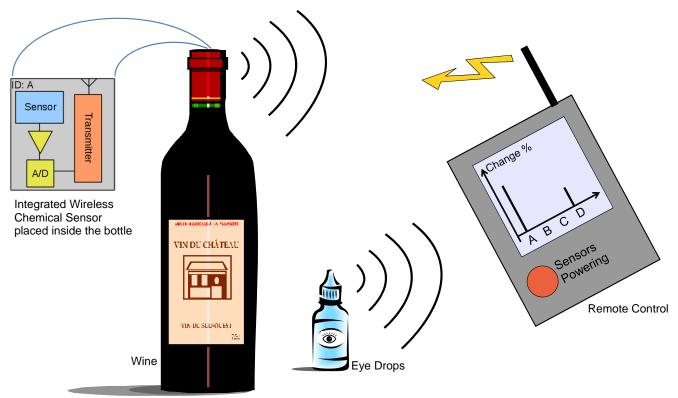
**Principle of the system.** Application to wine, medicine (eye drops...), etc. A remote control powers on the integrated chemical sensors placed inside the container. The sensors transmit their answer in a wireless way.
