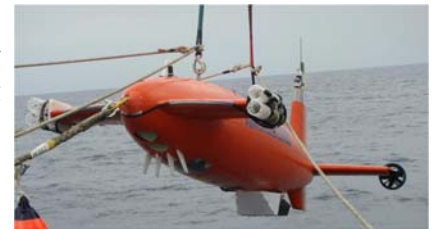
Aqua-Explorer 2000 for surveying hydrothermal vents
