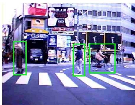
Fig 2. Pedestrian detection by monocular on-board camera
