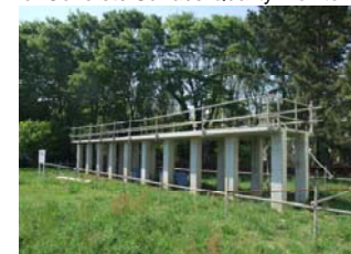
Mock-up of Rigid Frame Viaduct for Concrete Surface Quality Monitoring
