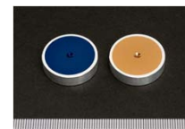
Al alloy machine components coated by the DLC films. The different colors are originated from the interference based on the film thickness, indicating the optical transparency of the DLC.
