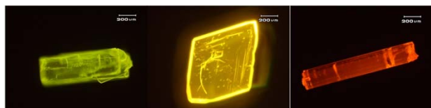
Luminescence of supramolecules – the same molecule, different packing mode.
