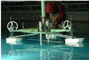
Comfortable boat with wave energy absorption suspension
