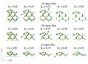
Deformation and fracture of Si nano-films were evaluated by DFT.
