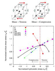
Ideal shear stress (ISS) under compression/tension, which is important to interpret experiments (e.g. nano-indentation tests), has been calculated. Response of ISS qualitatively differs. Note that compression always increases ISS in metals.
