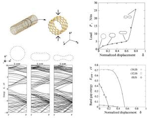
Mechanical properties and band gap of carbon nanotubes under radial compression have been evaluated. Compression can change electronic conductivity.
