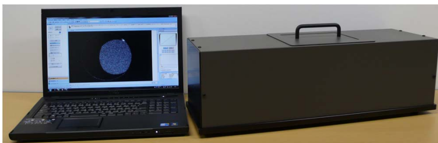
Fig.1 Speckle measurement tool prototype
