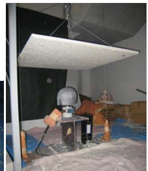
天井材落下実験 Drop experiment of ceiling panels
