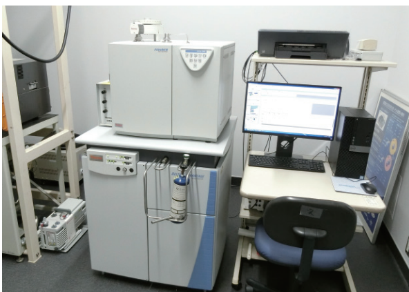
Mass spectrometer used for analyzing stable water isotope ratio
