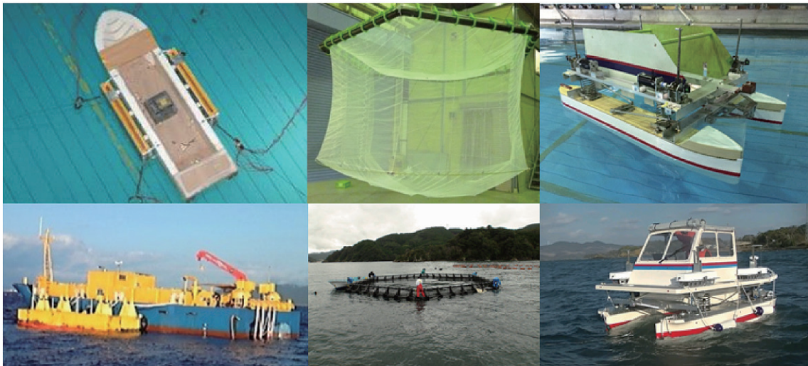
The water tank models (upper) and the prototypes or sub-scale models (lower) of an automated feeding platform (left), a submergible cage (center), a motion-controlled ship with wave energy harvester (right).
