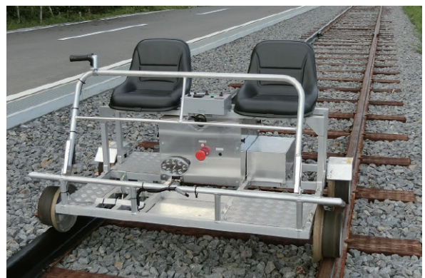
Test rail vehicle for the experiment of the automatic platooning
