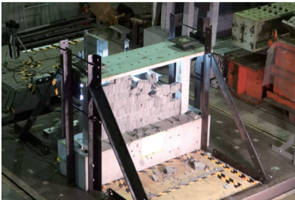
Unreinforced masonry wall collapse in non-rehabilitated specimen (left), less damaged, rehabilitated specimen (right)
