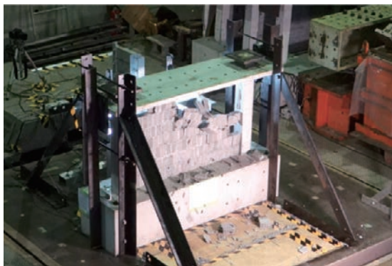
URM wall collapse in non-rehabilitated specimen (left), less damaged rehabilitated specimen (right)
