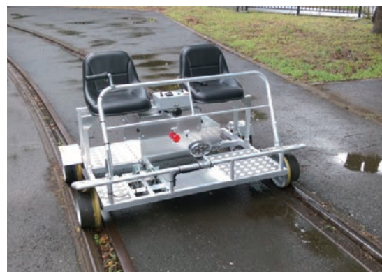
Test rail vehicle for the experiment of the automatic platooning
