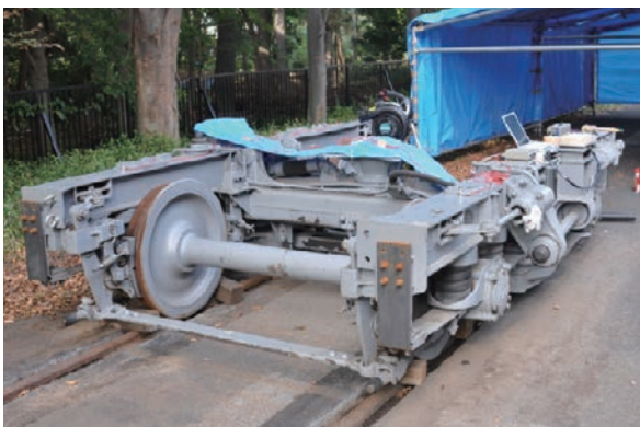
Experimental bogie for the detection of the irregularity on the rail
