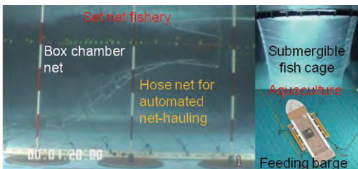
Automated flotation/submersion system of box chamber net and submersible fish cage with auto-feeding barge.
