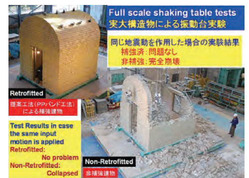
Full-scale shaking table test (Left: Retrofitted with PP-band, Right: Non-retrofitted)
