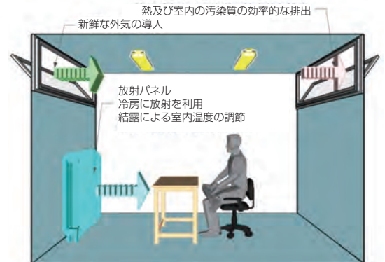
Concept of radiation panel cooling system with natural cross ventilation
