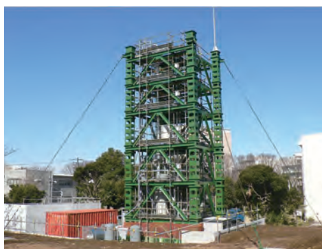
Experimental Apparatus of a large-scale triple-bed combined circulating fluidized bed consisting of riser, downer, and bubbling fluidized bed
