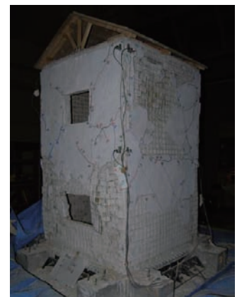
Model retrofitted with PP-bands
