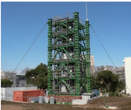
Experimental Apparatus of a Large-scale Triple Bed Combined Circulating Fluidized Bed Consisting of Riser, Downer, and Bubbling Fluidized Bed
