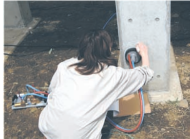
Estimation of surface air permeability
