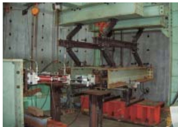
Whole view of Pseudo-dynamic test for two-story structure
