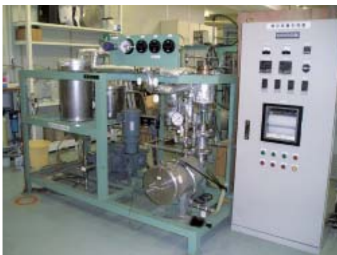
A laboratory scale apparatus of steam explosion treatment
