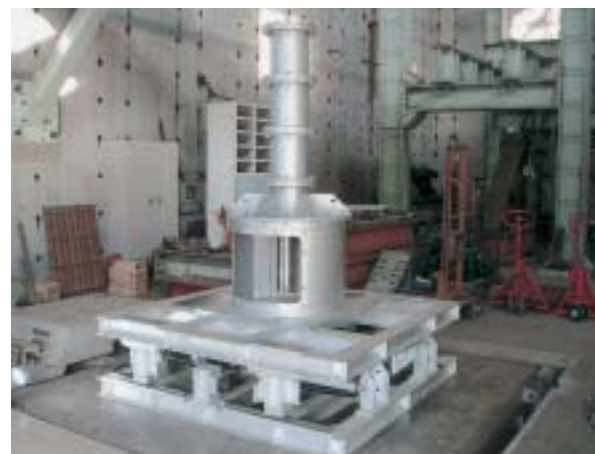
Excitation test for active-passive seismic isolation system
