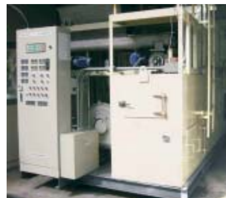
A test mobile process of super heated steam biomass pyrolysis.
