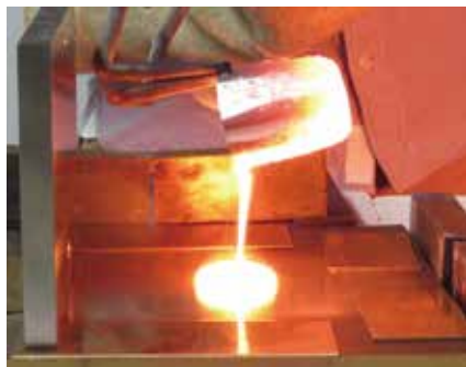
模擬廃棄物固化ホウケイ酸塩ガラスの熔融 Melting of simulated waste borosilicate glass
