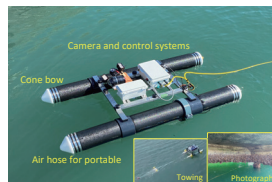
Reef-effect Observation around Marine Structure A portable monitoring system, MMC (Multi Over Catamaran)
