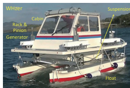
Wave Harmonizer (Yuya Bay, off Hiratsuka) Motion-controlled ship with wave energy harvester
