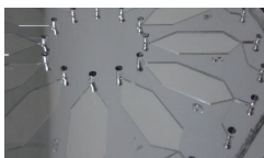
Microfluidic device for DNA purification
