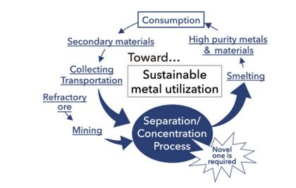
Tokoro laboratory conducts research to achieve an energy-efficient separation and concentration process that focuses on solid/solid separation and concentration without melting down the waste and ores. This process acts as a crucial “pre-treatment” or “intermediate treatment” in the overall metallurgical or hydrometallurgical processes that produce high-purity metals.
