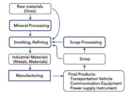
Kurokawa Laboratory aims to achieve processes that are energy-efficient, environmentally sound, and cost-effective by minimizing energy consumption in production and maximizing the recovery of target metals to reduce waste generation.
