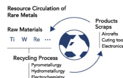
Okabe laboratory is dedicated to developing innovative, high-efficiency, and environmentally sound recycling technologies for rare metals such as titanium, which is anticipated to see increased demand as a structural material; tungsten and cobalt, indispensable in tool materials; rhenium, which is used in nickel-based superalloys; and platinum group metals found in automotive exhaust catalysts.
